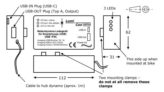
Fig. 5: Dimensions and Interfaces
