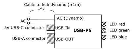
AC: input, connection to hub dynamo, two-core cable, 1m, black, fixed to harvester USB-IN: USB-C plug, input 5V, for usage with attached mains charger USB-OUT: output, USB-connector type A, 5V / 1.5A max.
