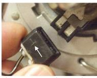
2) Disconnect and remember the wire which was connected to GND (symbol  $\perp^{**}$ )
