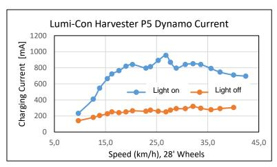
Fig. 3: Charge current and power at a battery voltage of 8V vs. speed, typical hub dynamo (Shimano)
