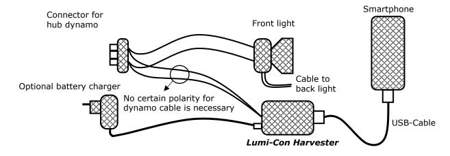
Fig. 6: Connecting the Lumi-Con-Harvester
