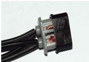
5) Strip isolation for all wires by 20-25mm
