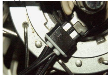
6) Twist wire pairs and cut stripped wires exactly to 18mm
