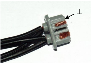
7) Pull in the two wire ends into connector and care for polarity (GND ⊥, see 2)) *
