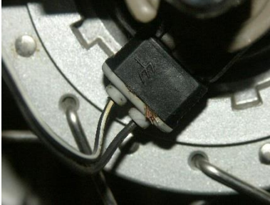
1) Look for connector at wheel hub
