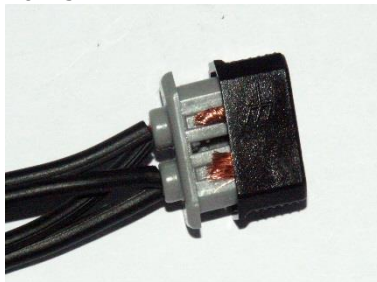
8) Slide on connector cap
