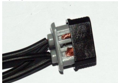
5) Strip isolation for all wires by 20-25mm
