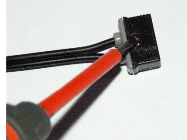
3) press flap with suitable tool (e.g. small screwdriver)
