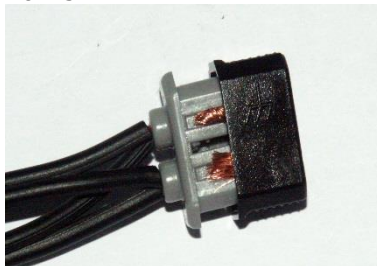
5) Strip isolation for all wires by 20-25mm
