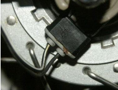
1) Look for connector at wheel hub
