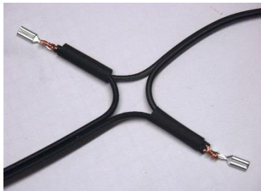
4) Shift the hose on the cable as shown and solder the flat plug, do not heat the hose.
