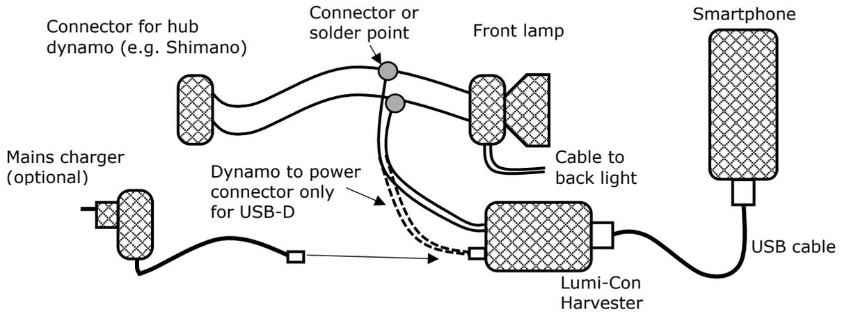
The *Lumi-Con-Energy-Harvester* must be connected directly to the hub dynamo cable. Do not connect to the back light cable. **Please remove the plastic clips at the batteries inside the harvester before starting!** Beside the method using the dynamo connector you can directly attach to the dynamo cable. Here two examples:
