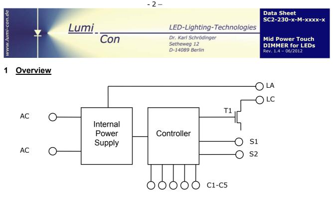
The DIMMER module can be connected directly to mains voltage (AC 230V, 50Hz) without using a transformer. It can drive up to 72 white LEDs at a current up to 100mA. The LED power is controlled via the touch pads (S1, S2) or the control pins (C1 ... C5). A Sensor Pad is a simple metal surface electrically connected to S1/S2. The controller incorporates DIMMER and ON-/OFF operation.
