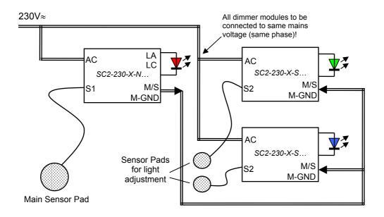
Lumi-Con dimmers (Normal and Master version) provide a 1kHz signal at the Master output (M/S OUT) with an amplitude of about 3V when the light is switched on. This signal is able to switch on a Slave module (SC2-230-X-S...). Maximum two Slave modules can be driven from a Master module. All DIMMER-Modules interconnected through M/S and M-GND must be attached to the same mains supply (same phase).
